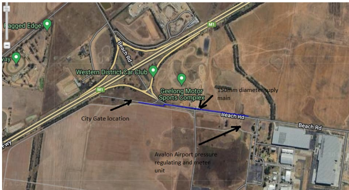
Figure 11 – Existing Gas Network (provided by Ausnet)
