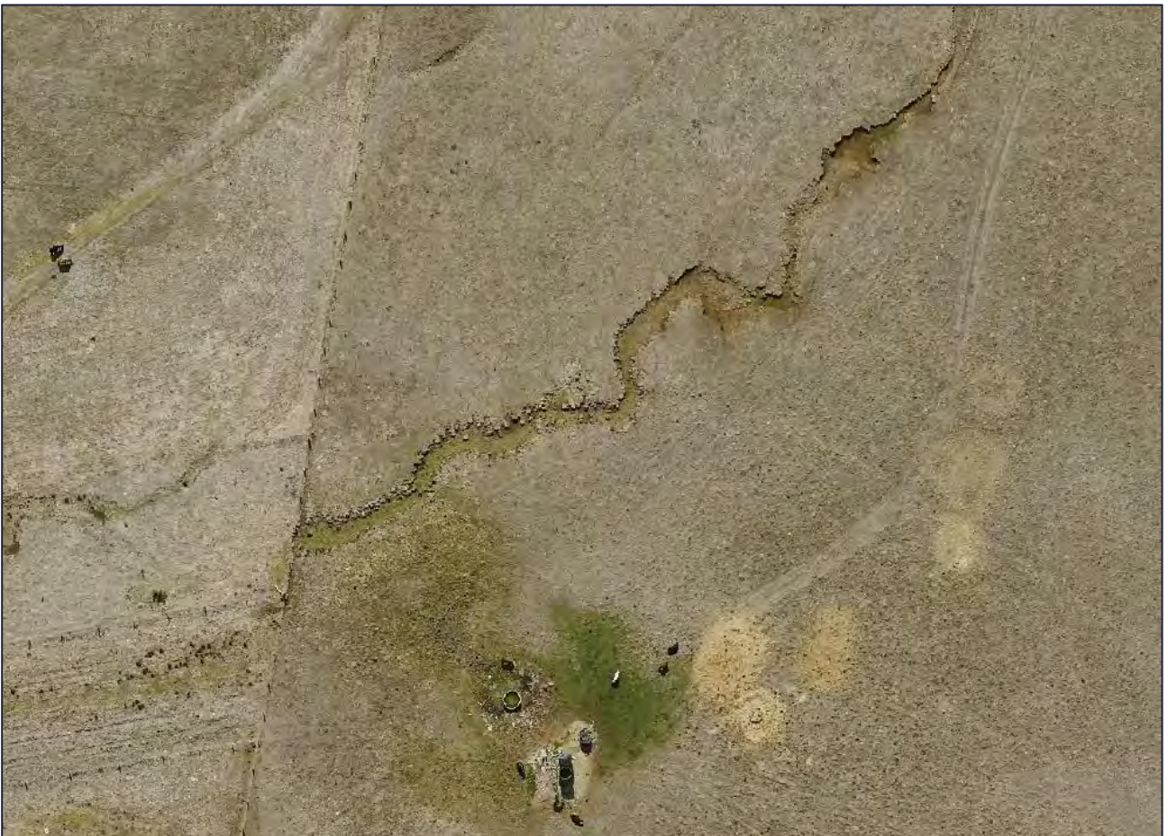
Figure 3-15 Lack of riparian vegetation and agricultural activities resulting in surface erosion, near the upstream end of the PSP area
