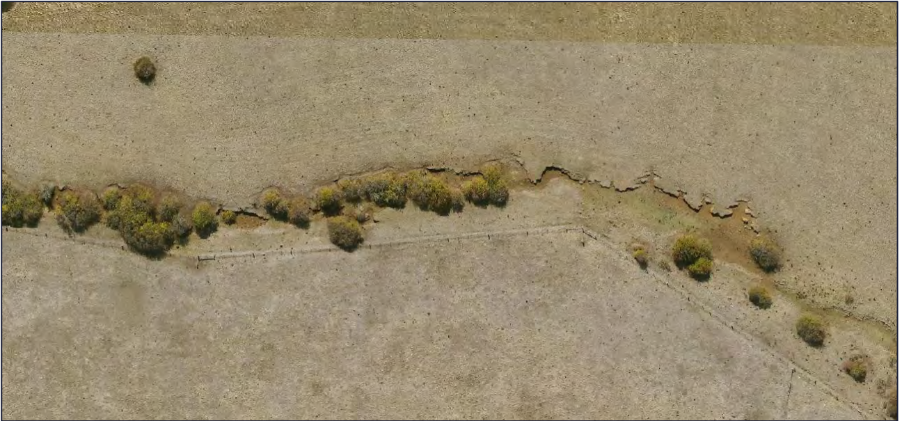
Figure 3-14 Lack of riparian vegetation and agricultural activities resulting in surface erosion, approximately chainage 660 from Aberline Road
