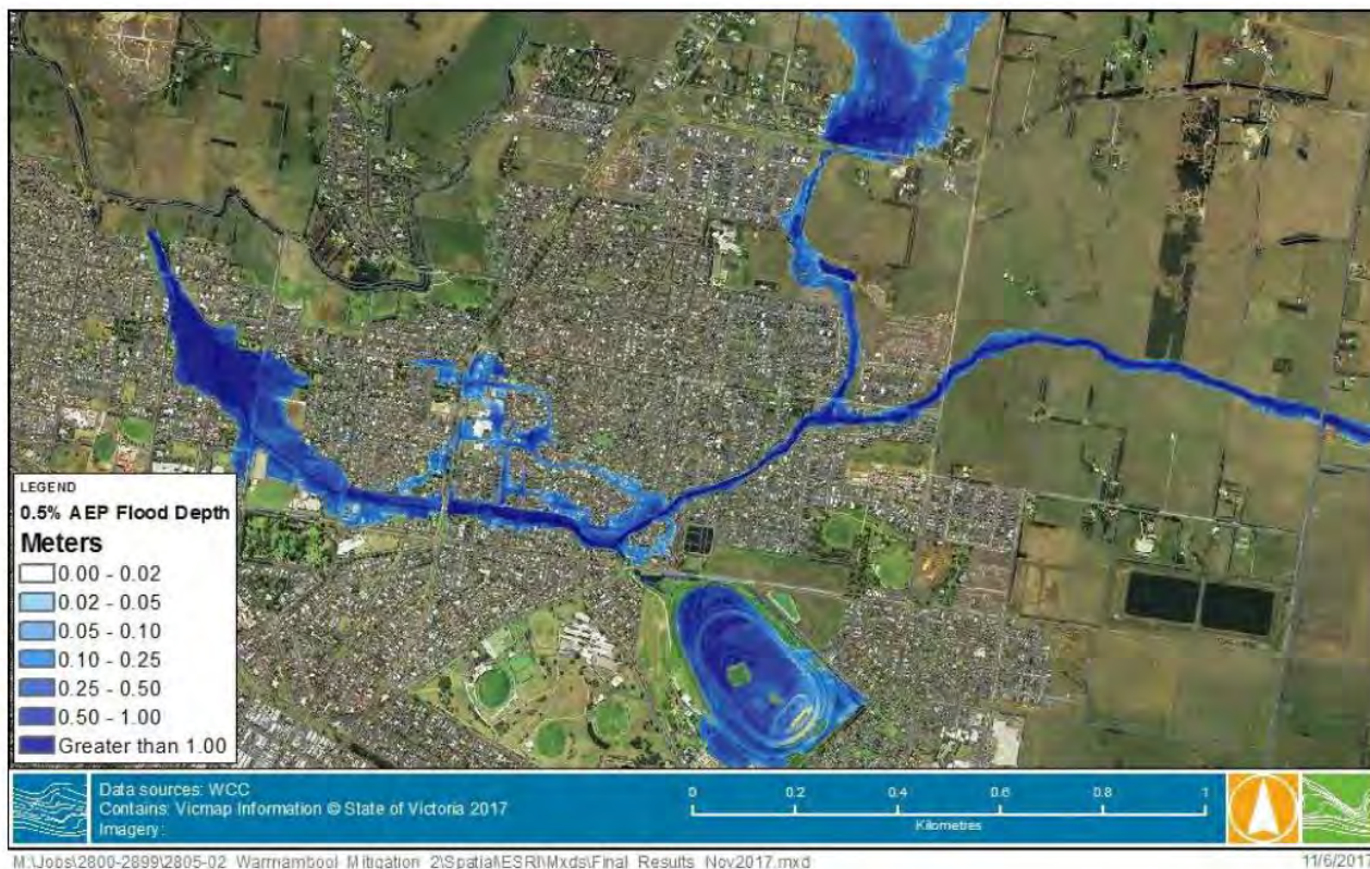
Figure 4-2 Water Technology 2017 1% AEP Flood Modelling Outcomes for Design Conditions
