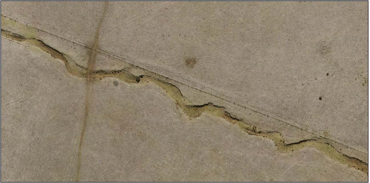
Figure 3-16 Lack of riparian vegetation and agricultural activities resulting in surface erosion, approximately chainage 1220 from Aberline Road
