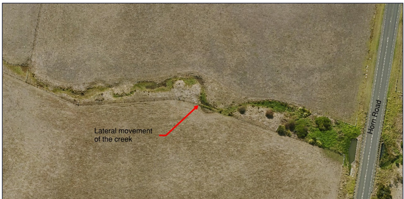
Figure 3-19 Lateral movement of the creek and the formation of pools and riffles downstream of Horne Road
