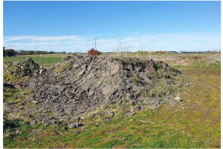
Photograph 49: View of a stockpile around the shed. Soils consisted of a clayey silt with large amounts of crushed asphalt. In the right of image some rusted farm equipment can be seen buried within a stockpile.
