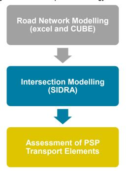
Traffic generation and distribution inputs are used to develop an origin-destination (O-D) matrix in excel. CUBE software is then used to assign the O-D matrix to the network resulting in network traffic volume plots and turning movement data.
