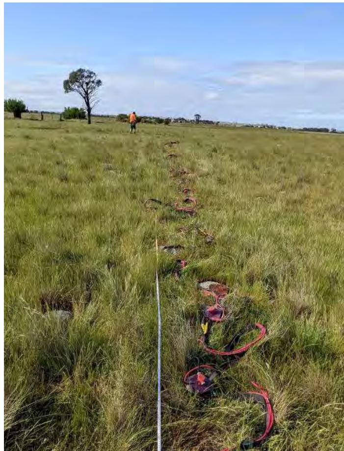
Figure 5: Example of a seismic line survey configuration.
