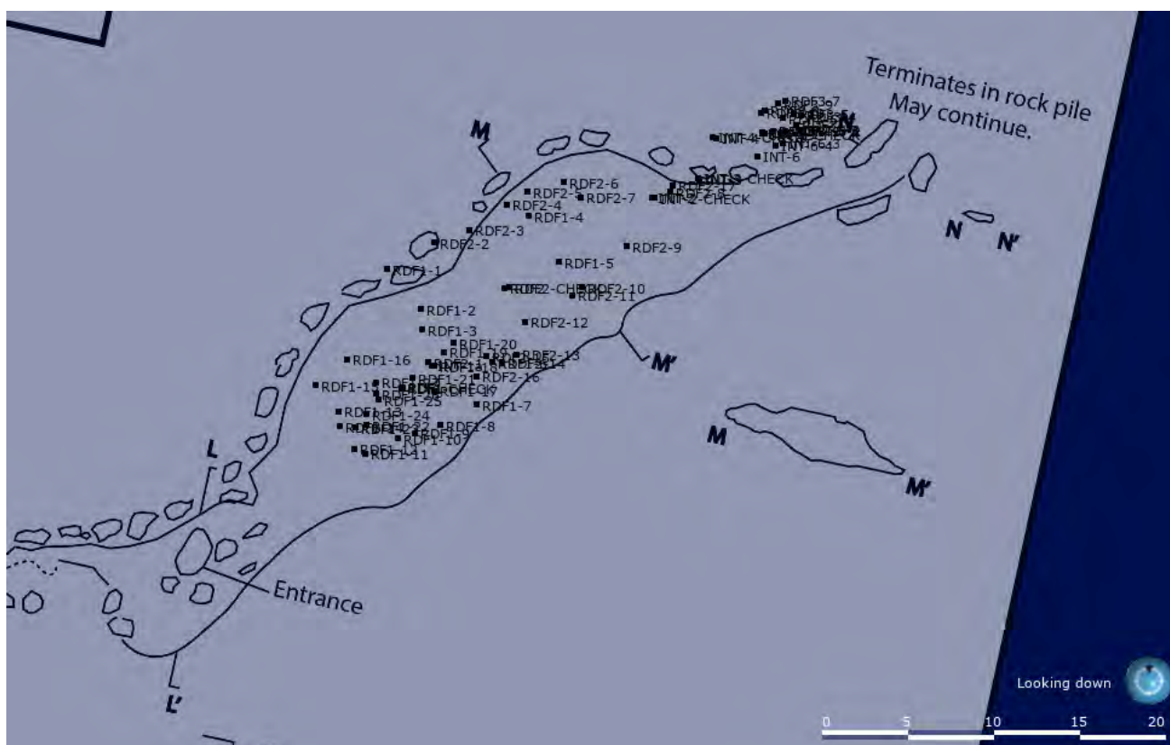
Figure 2: Disto measurements relative to RDF points plotted on VSA 1969 speleological survey
