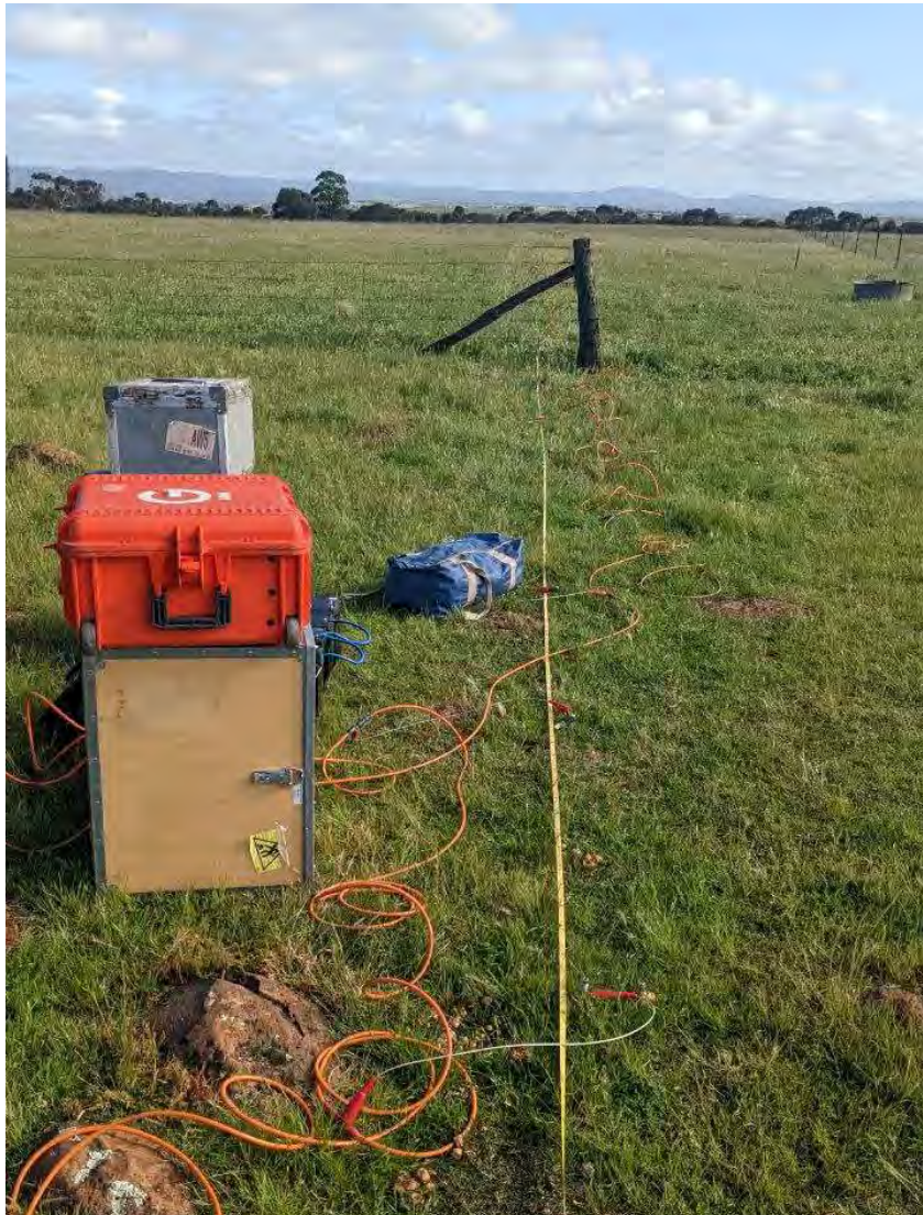
Figure 6: Example of an ERT survey configuration.
