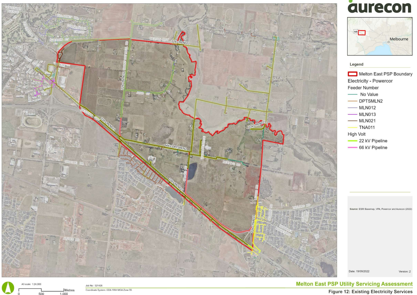
Figure 12 Existing Electricity Services
