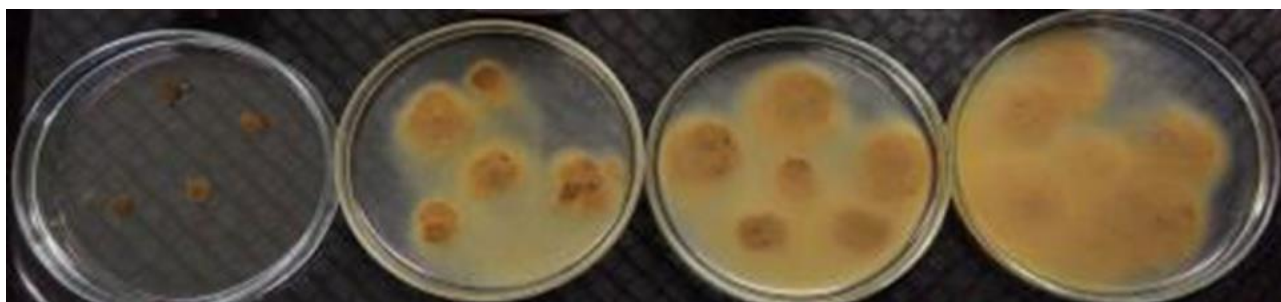
Figure 2-1. Examples of soil aggregates subject to the Emerson Aggregate Test, showing nil dispersion on the left with increasing levels of dispersion to the right (Armstrong 2019).
