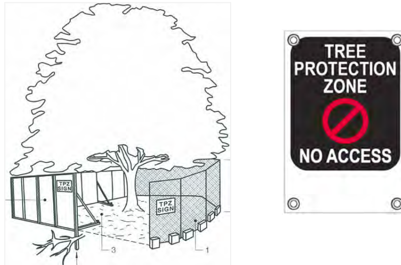
Figure 1. Above left - Example of TPZ fencing above right -Example of TPZ signage.
