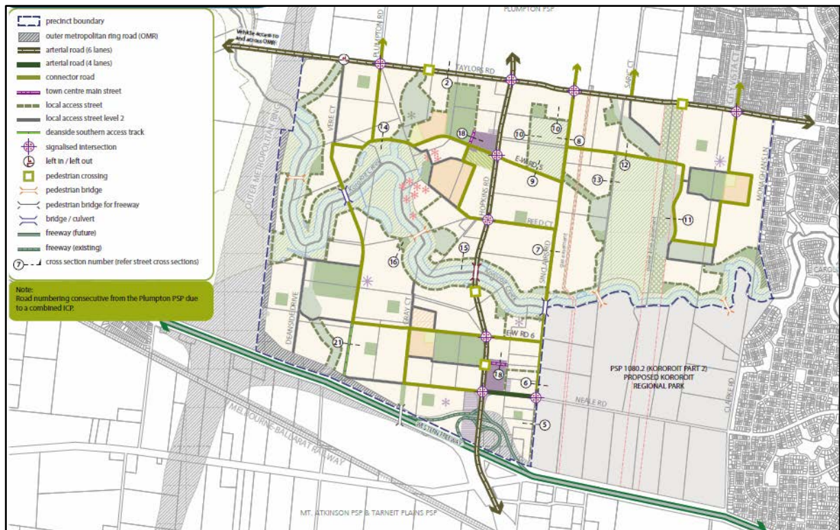
Figure 2: Kororoit PSP Plan 8 - Road Network Plan
