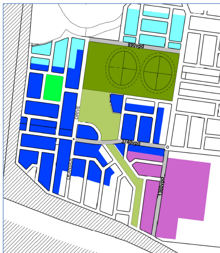
Figure 2: Predicted traffic volumes resulting from road network design
