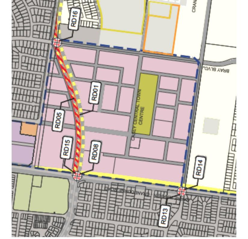
Extending south from The Strand the street is located between two high points within the precinct, and is required in this location to facilitate the transfer of stormwater between drainage catchments (see **Section 4**). This location results in a slight curve in the street to enable a connection with The Strand to the north.
