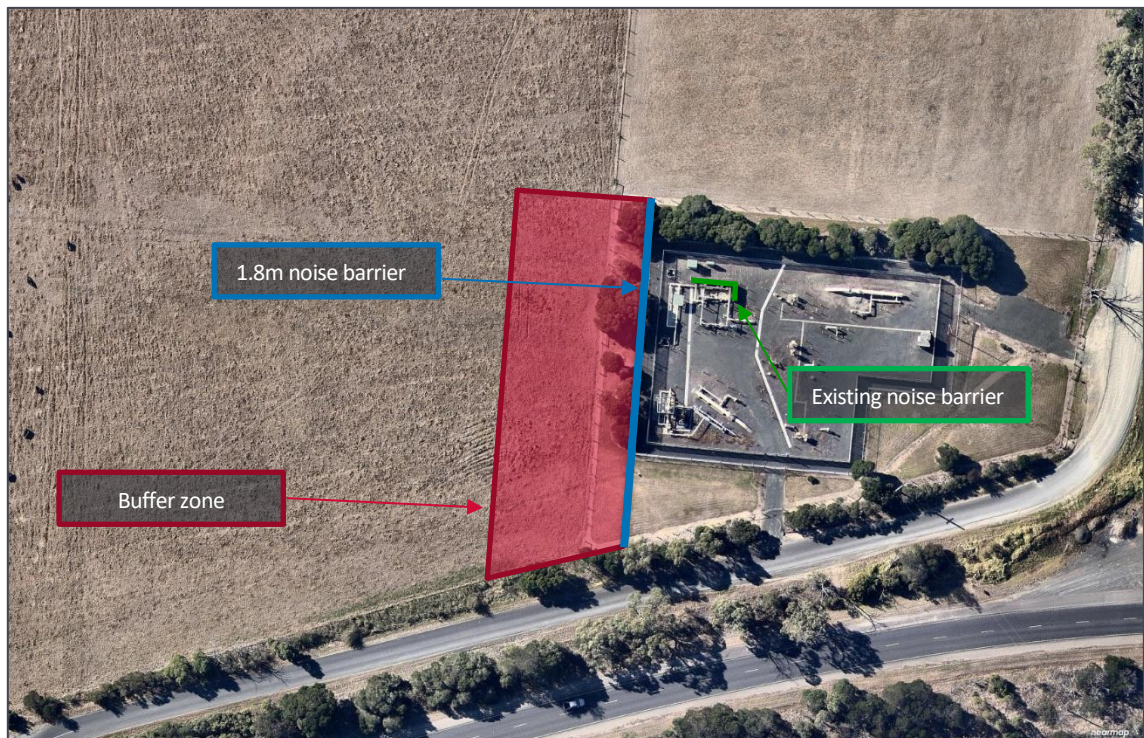
Figure 5: Buffer distance and/or recommended barrier location
