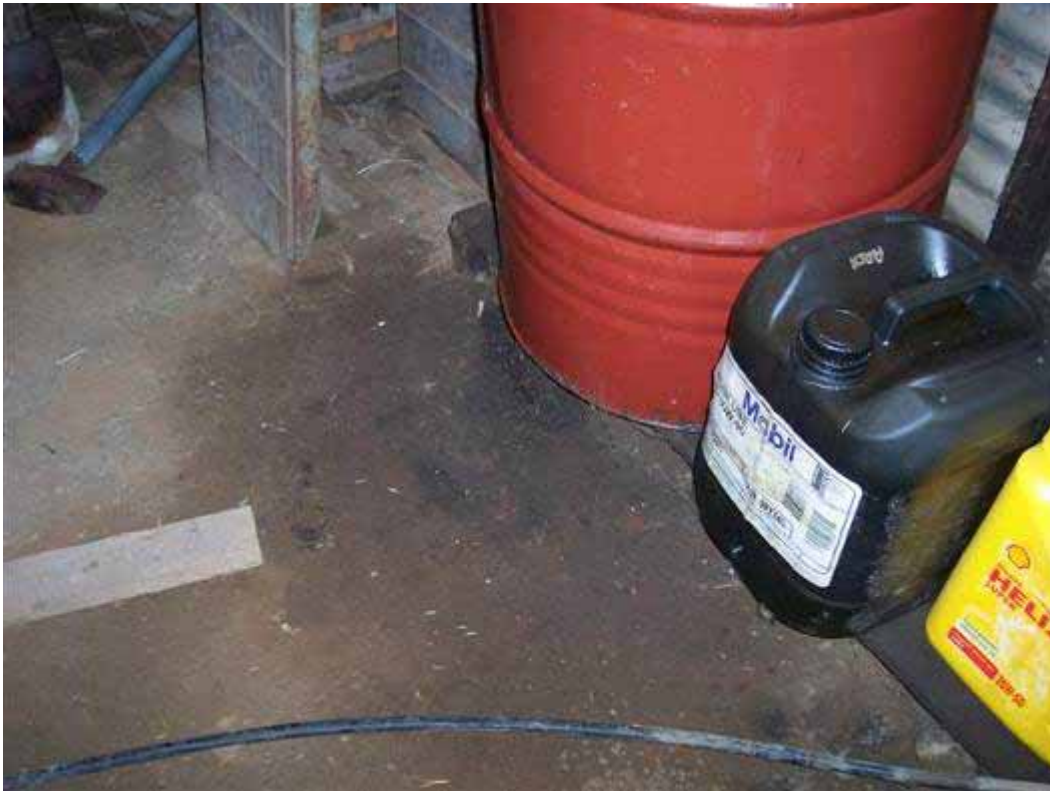
Plate P17: 185 Verney Road - Close-up of possible hydrocarbon staining
