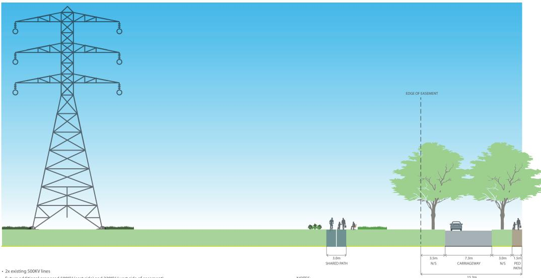
• Future additional proposed 500KV (east side) and 220KV (west side of easement).
