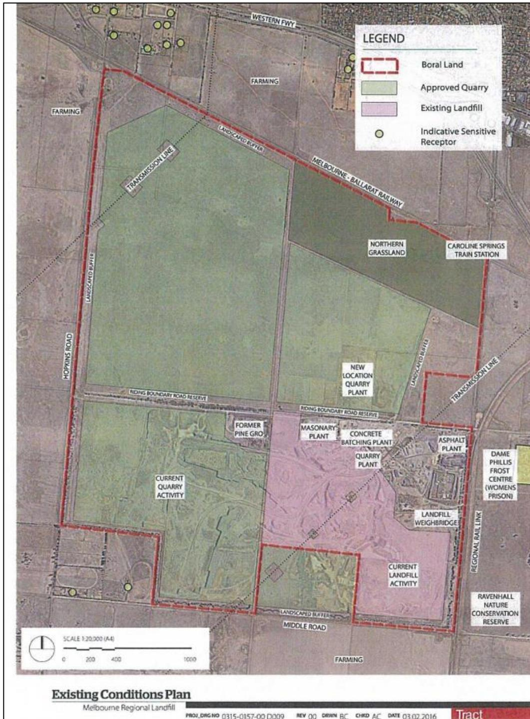
29. The above figure also provides a good indication of the existing nearest residential receivers to the quarry, located to the south-west and the north-west. There is also a prison to the direct east of the site, which is a noise sensitive receiver.
